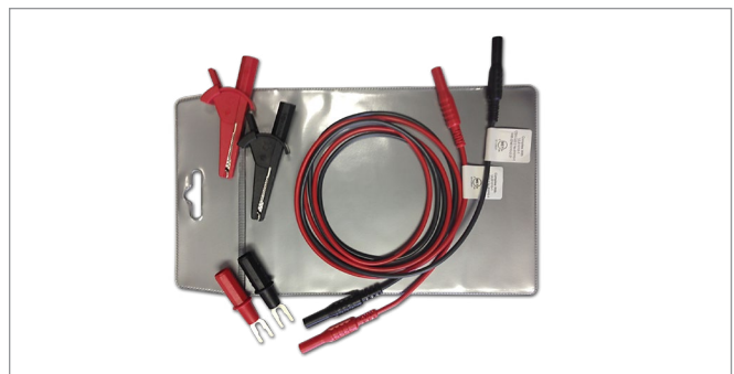
2280-TEST-LEAD: Power Supply Test Lead Kit, 1000V, 20A Rating: Contains 122cm (4ft) of cable, spade lug adapters, and alligator clips
