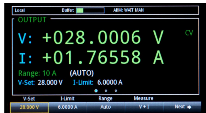
Figure 3. Adjust voltage, current, the current range, the measurement mode, protection levels, and other functions from the home screen.
